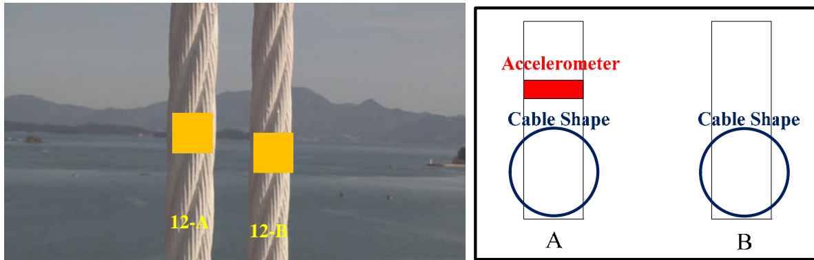
Fig. 6 Sensor installation position
