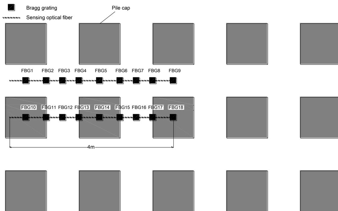
Fig. 2 Location of optical fibers and Bragg gratings relative to the pile caps
