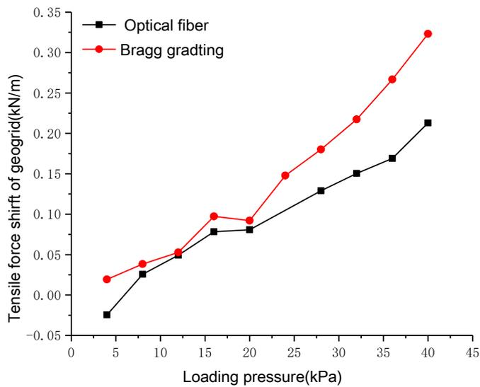
Fig.5 The tensile force in geo-grid at the center of the embankment
