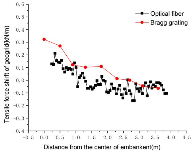
Fig.4 Tensile force shift of geo-grid at the static load of 40kPa
