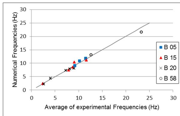
Figure 7 – Numerical Frequencies Vs Average of Experimental frequencies, after the model adjustment
