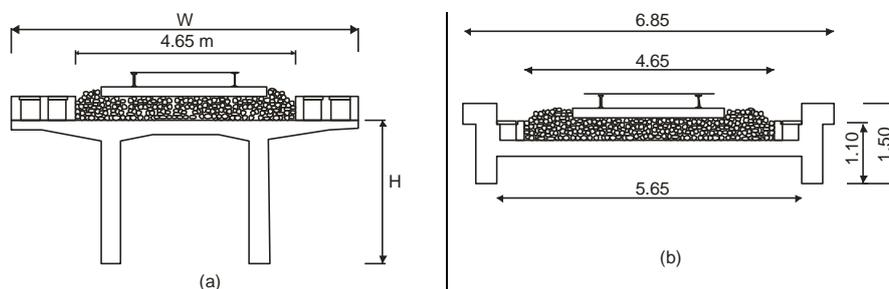
Figure 2 – Sketch of typical cross sections. (a) B20, B15 and B5; (b) B58A
