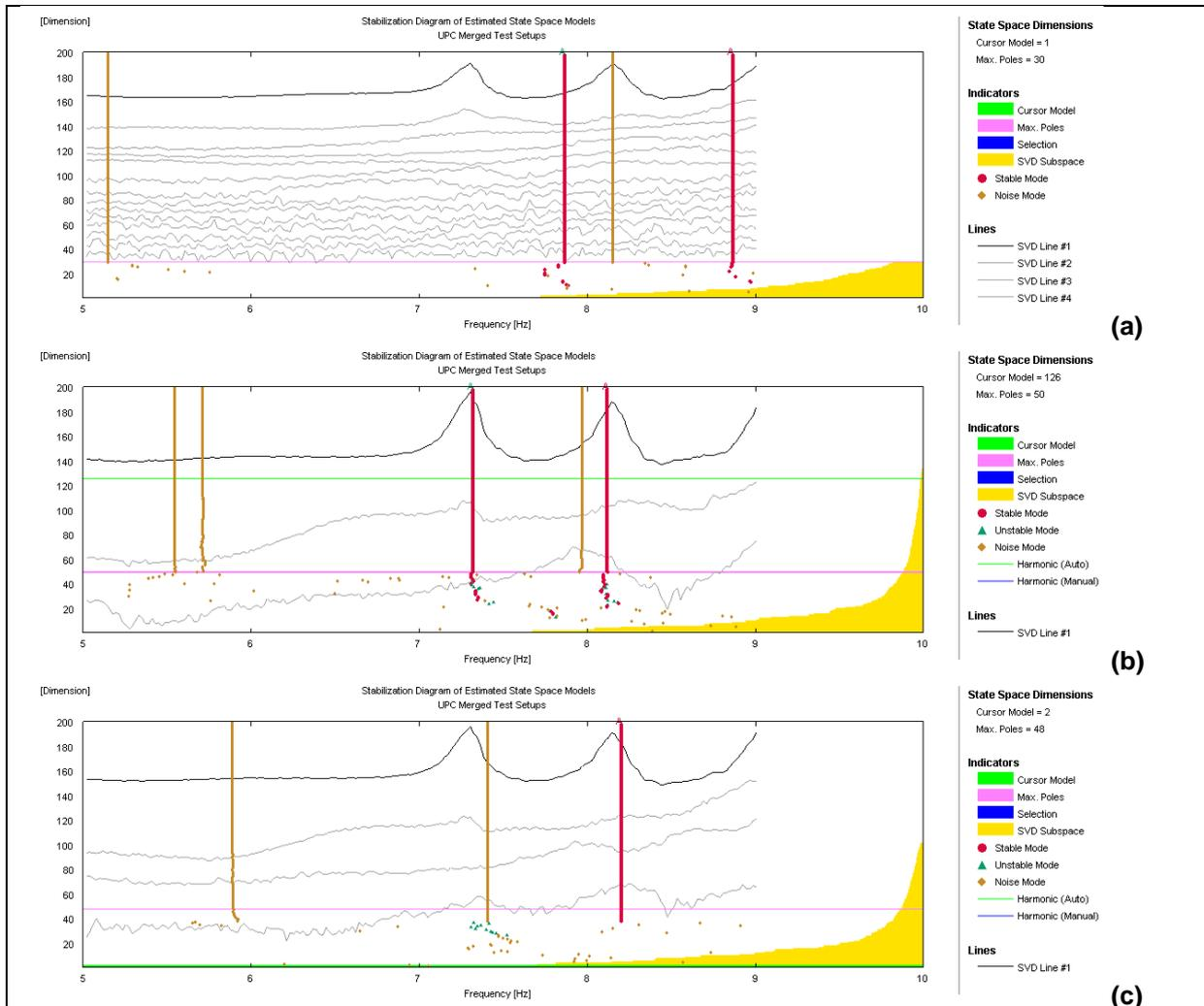
Figure 4 – Stabilization diagram in a frequency range of 5 to 9 Hz, for tests with drop weight in Bridge 20, considering: a) without projection channels; b) 3 projection channels and c) 4 projection channels.
