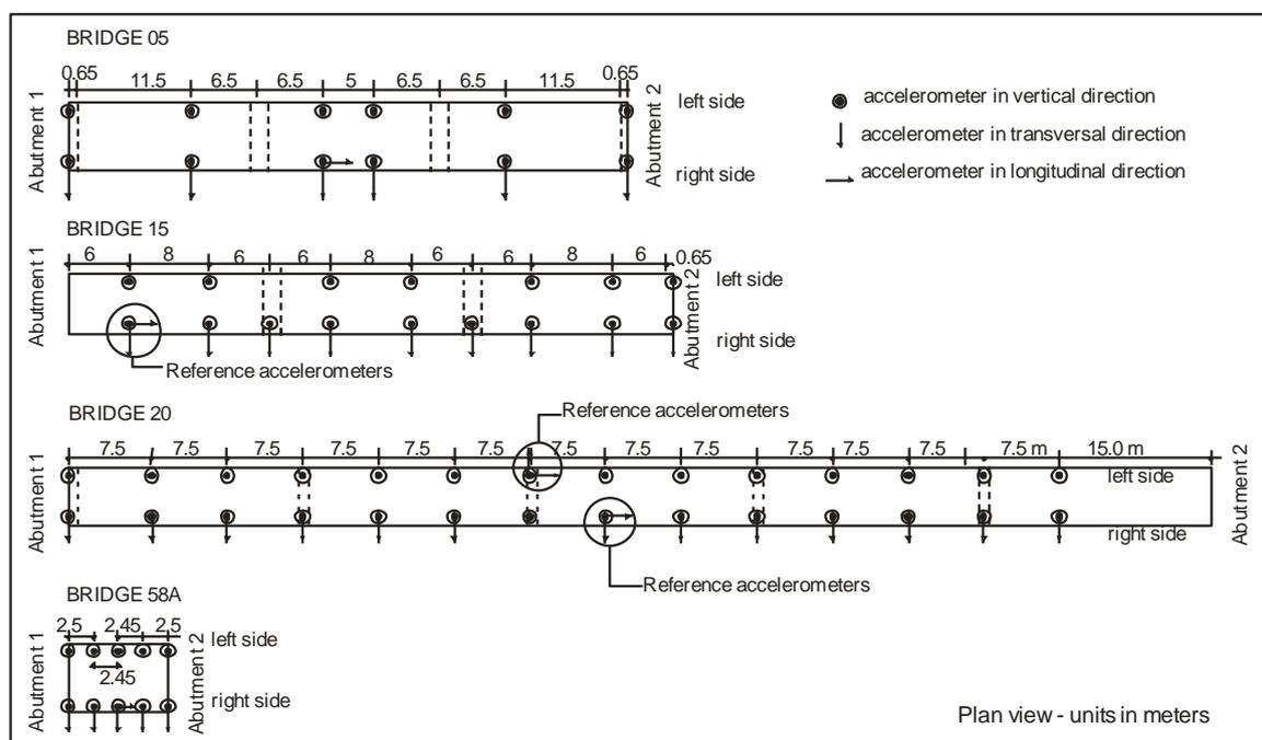
Figure 3 – Accelerometer layout
