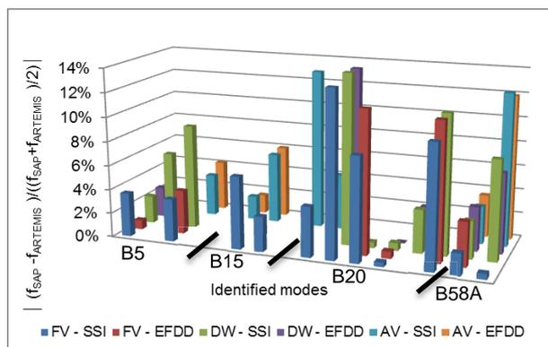
Figure 6 –Matrix of Variation between numerical and experimental frequency values for each type of records and method of analysis for all bridges.
