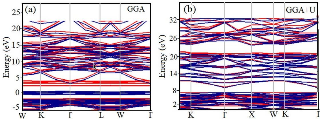
Fig. 2 Band diagram of  $\text{FeAl}_2\text{O}_4$  taken from (a) GGA and (b) GGA+U calculations.
