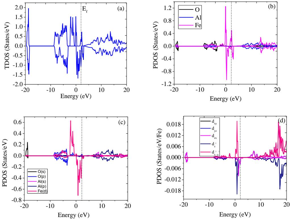
Fig. 3 Total and partial density of states of  $\text{FeAl}_2\text{O}_4$  calculate using GGA:PBE approximation.
