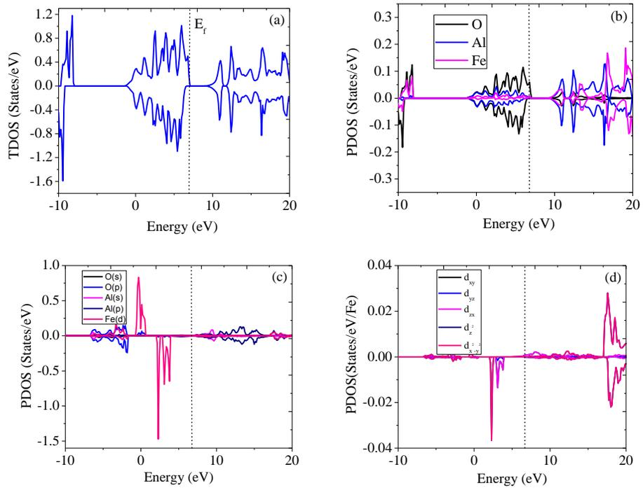
Fig. 4 Total and partial density of states of  $\text{FeAl}_2\text{O}_4$  calculate using GGA+U approximation.
