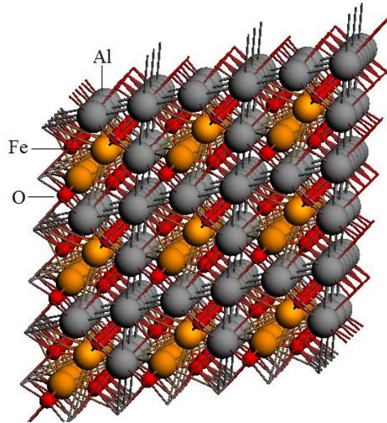
Fig.1 Diagram of  $\text{FeAl}_2\text{O}_4$  spinel structure where Fe atom occupied tetrahedral sites and Al atom occupied octahedral sites.
