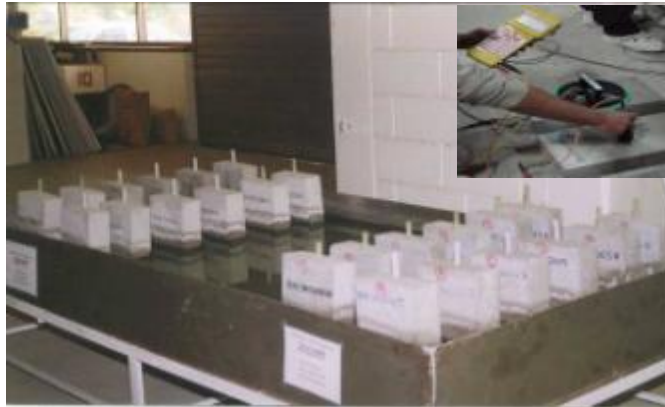
Fig.2. Test setup of Corrosion Rate Test (Lollipop Test)
