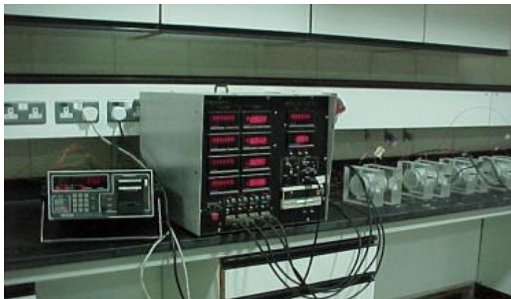
Fig. 3. Test setup of electrical indication of Concrete’s Ability to Resist Chloride.
