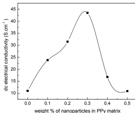
**Fig. 2** DC electrical conductivity as a function of Nanoparticle loading percentage
