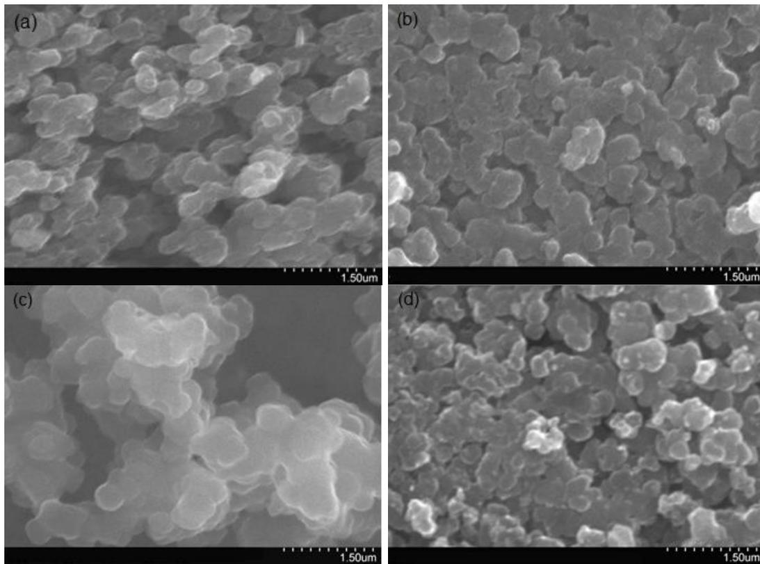
**Fig. 3** SEM micrographs of (a) PANI (b) PNC-0.1% (c) PNC-0.3% (d) PNC-0.5%
