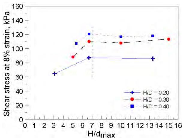
Fig. 11 Shear stress at 8% versus  $H/d_{max}$
