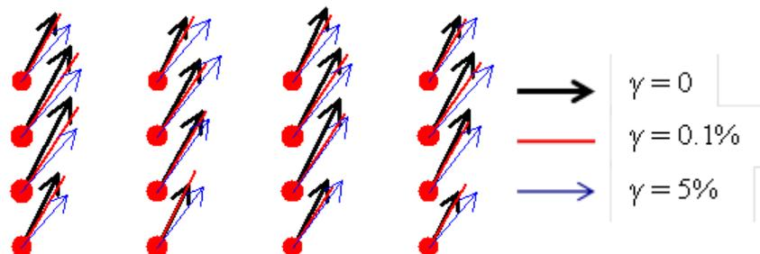
Fig. 6 Rotation of principle stresses in the core of NGI model
