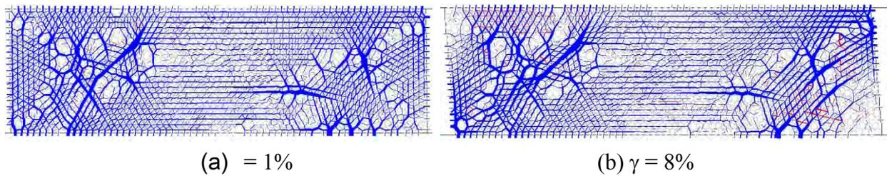
Fig. 7 Force chains at two shear strain levels
