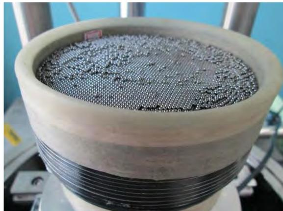
Fig. 2 Uniform steel ball specimen for DSS testing
