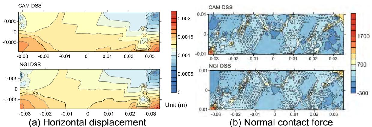
Fig. 8 Comparison of particle responses between NGI and CAM DSS models
