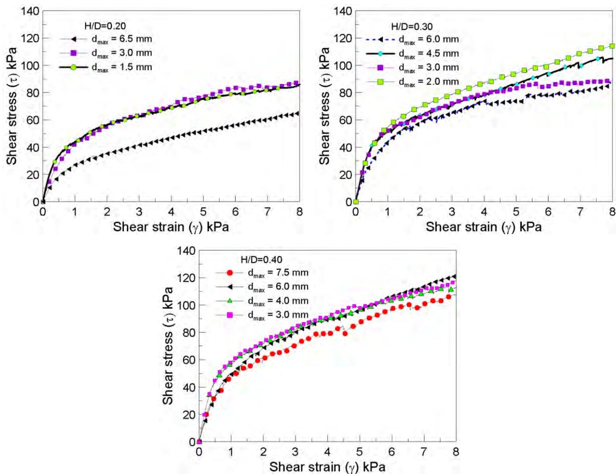
Fig. 10 DEM simulation results for different maximum particle sizes and H/D ratio
