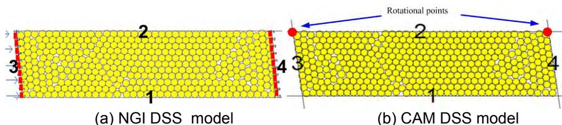
Fig. 4 Direct simple shear DEM models
