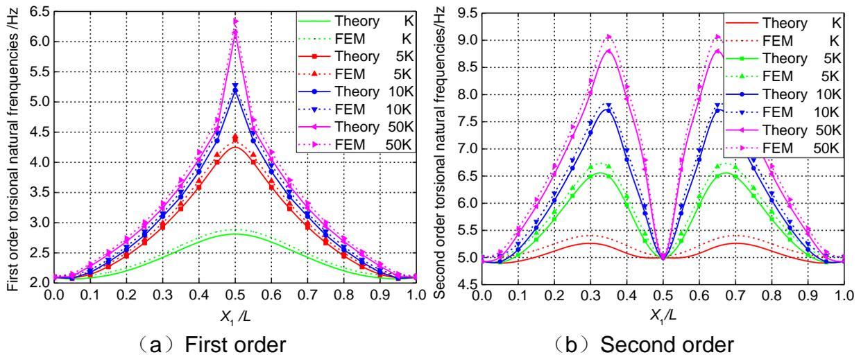
Fig.6 The lowest two torsional natural frequencies of the coupled system with H-section hanger and wind-resistant cables in different locations versus  $\varepsilon$
