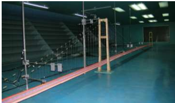
d) Full bridge aeroelastic tests
