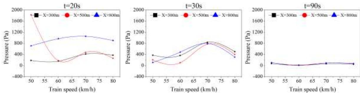
Fig.7 Pressure variation with train speed: (a) t=20s; (b) t=30s; (c) t=90s
