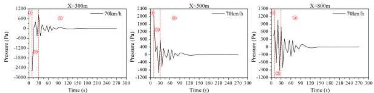
Fig.4 Pressure variation with time of three typical locations
