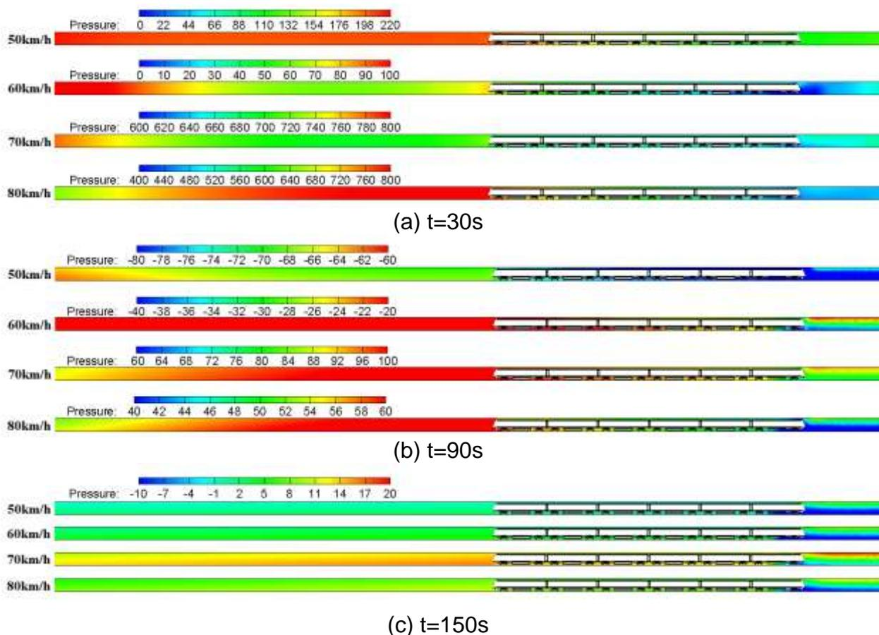
Fig.6 Pressure distribution in different train speed: (a) t=30s; (b) t=90s; (c) t=150s
