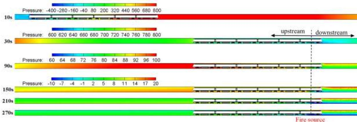
Fig.3 Pressure around train varying with time
