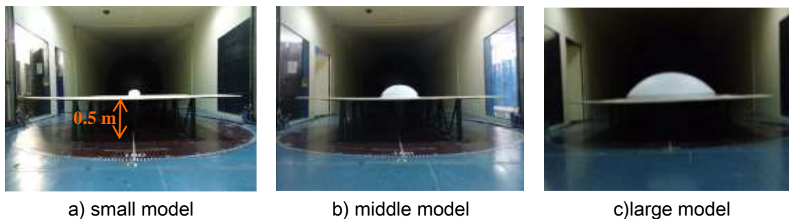
Fig. 1 Pictures of wind tunnel tests in smooth flow
