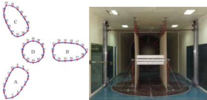
(a) Sectional tap arrangement (total 54 taps) (b) Picture of 2-D sectional model setup
