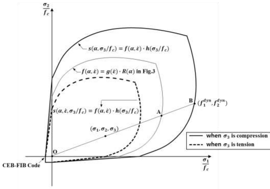
Fig. 4 Strain rate dependent triaxial failure envelope
