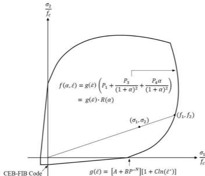
Fig. 1 Strain rate dependent bi-axial failure envelope
