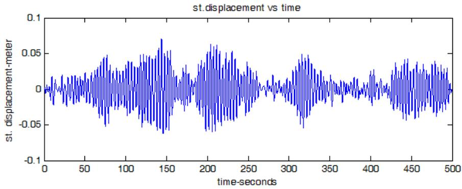
Fig.7 Along-wind responses with ATMD ( $\mu_{AP}=0.1$ , rms=0.0219)
