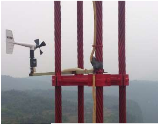
Fig 3 Anemometer arranged on the cable
