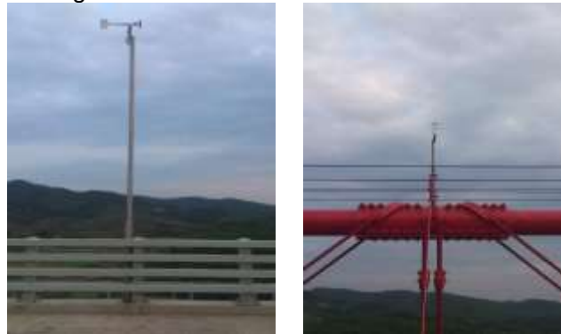
Fig2 Anemometer arranged in the middle span
