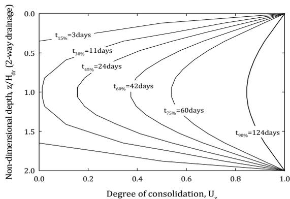
**Fig. 6** Projected development of the degree of consolidation isochrones
