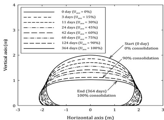
**Fig. 5** Geotextile tube geometric shapes during the consolidation process
