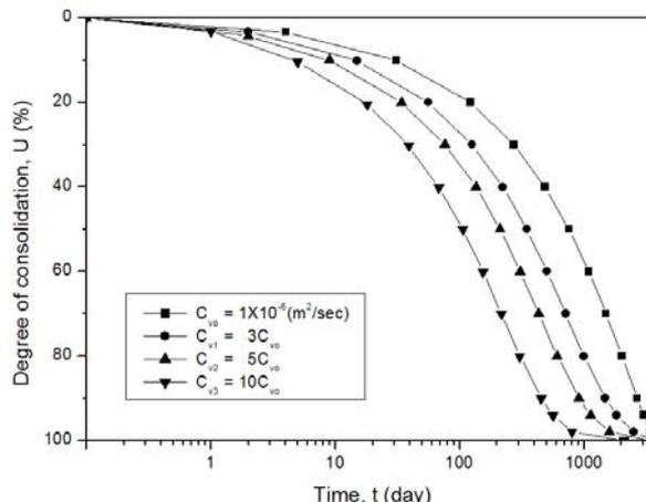
**Fig. 13** Degree of consolidation and time comparison with increasing  $C_v$
