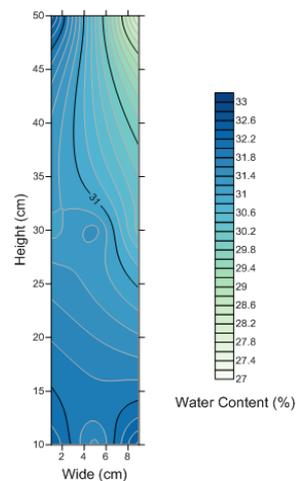
**Fig. 11** Water content of nonwoven material
