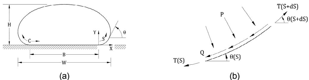
Fig. 1 (a) Tube cross-section and (b) forces acting on the differential element (after Plaut and Suherman 1998)
