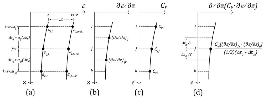
**Fig. 3** (a) Variation of strain  $\epsilon$  with depth, (b) first derivative of strain, (c) variation of strain  $C_v$  with depth and (d) second derivative of strain
