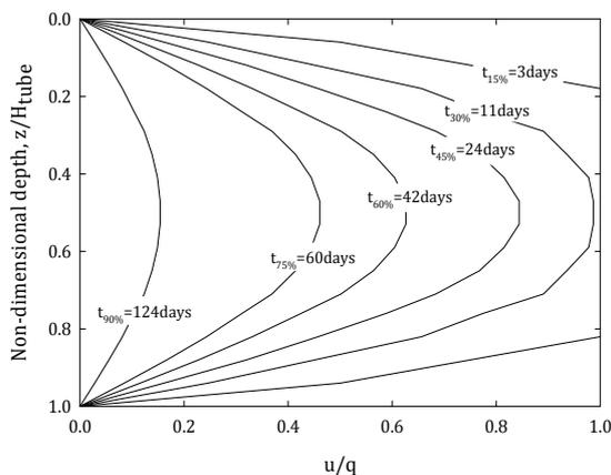
**Fig. 7** Projected development of excess pore water pressure isochrones
