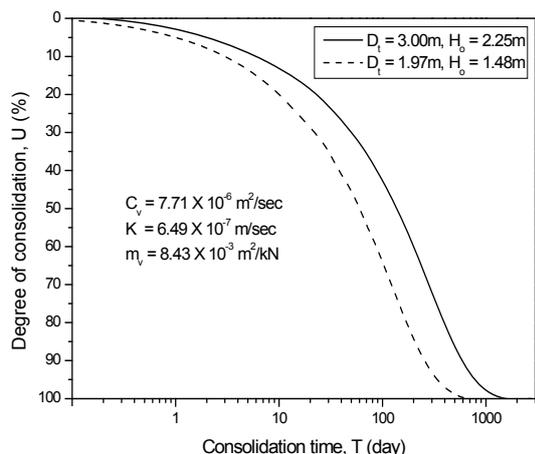
**Fig. 12** Degree of consolidation with respect to time with different diameters
