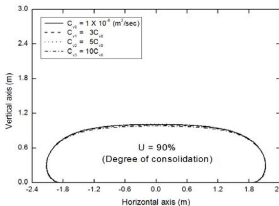
**Fig. 14** Geotextile shape comparison with increasing  $C_v$  ( $U=50\%$ ,  $90\%$ )
