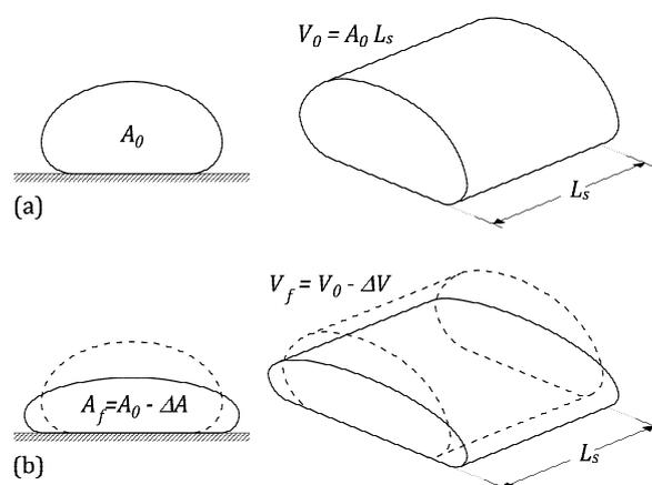
**Fig. 2** Geotextile tube segment: (a) Final filling state and (b) final consolidation state
