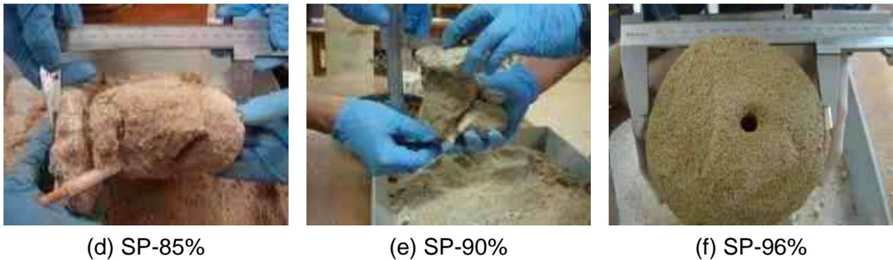
Fig. 4 Results of bio-grouting of SP specimens according to ground conditions
