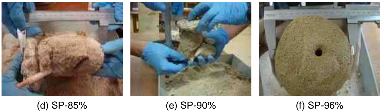
Fig. 4 Results of bio-grouting of SP specimens according to ground conditions
