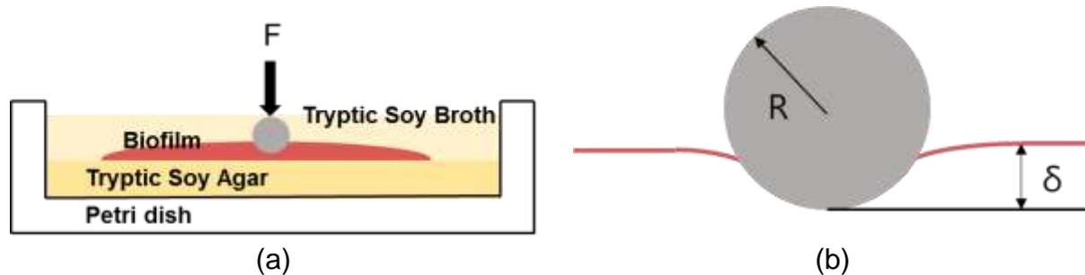
**Fig. 1.** (a) A schematic diagram of the sample, and (b) a schematic diagram of the Hertzian contact model for a spherical indenter on a half-elastic plane.
