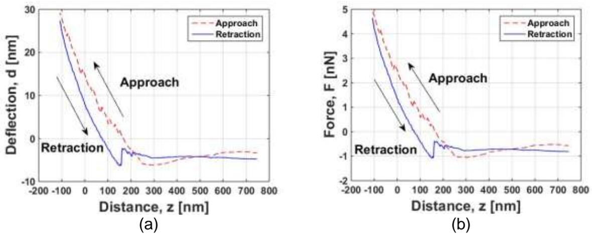
Fig. 2. (a) Deflection-distance result, and (b) force-distance result.
