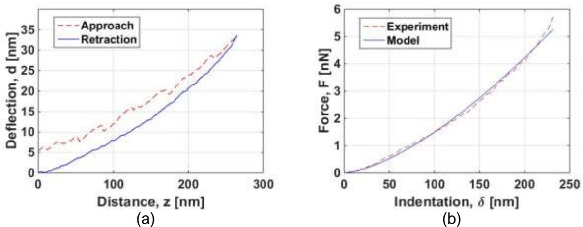
Fig. 3. (a) The deflection-distance curve extracted, and (b) The force-indentation curve for model fitting.
