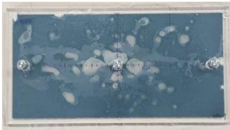
Fig. 8 An example of air bubble occurrence in the grouted fracture.
