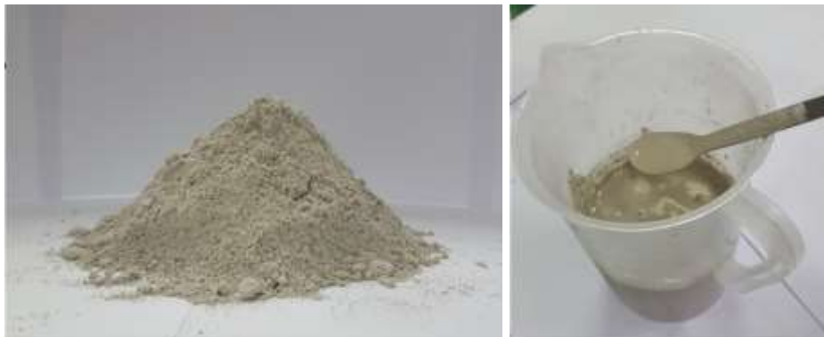
Fig. 3 Material (micro cement) used for grouting injection.
