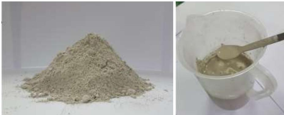
Fig. 3 Material (micro cement) used for grouting injection.
