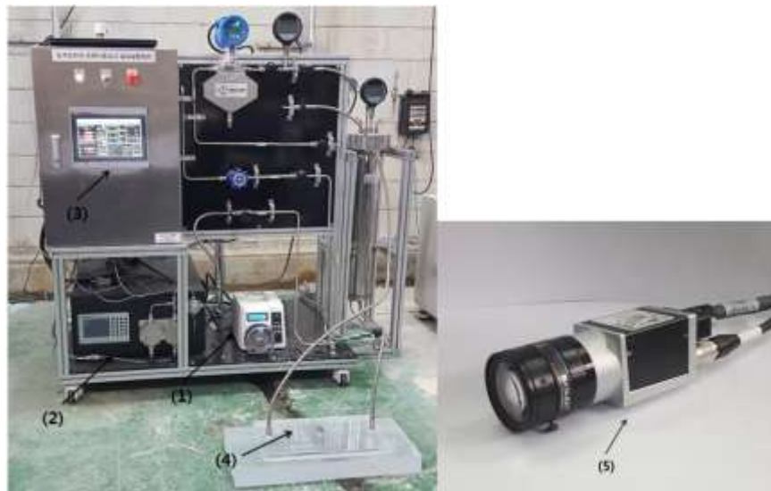
Fig. 1 Picture of experimental set-up. (1 – Syringe pump; Accurate high-pressure pump; 3 – Multichannel data acquisition and control box; 4 – Test section; 5 – Digital camera).
