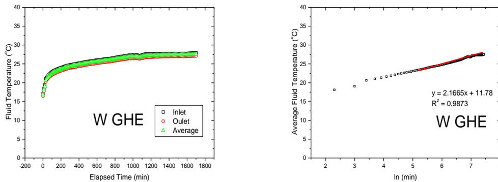
(a) Temperature distribution vs. time (b) Temperature distribution vs.  $\ln t$
