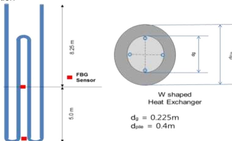
Fig. 2 Dimensions of the energy pile with the W shape (Yoon *et al.* 2014)
