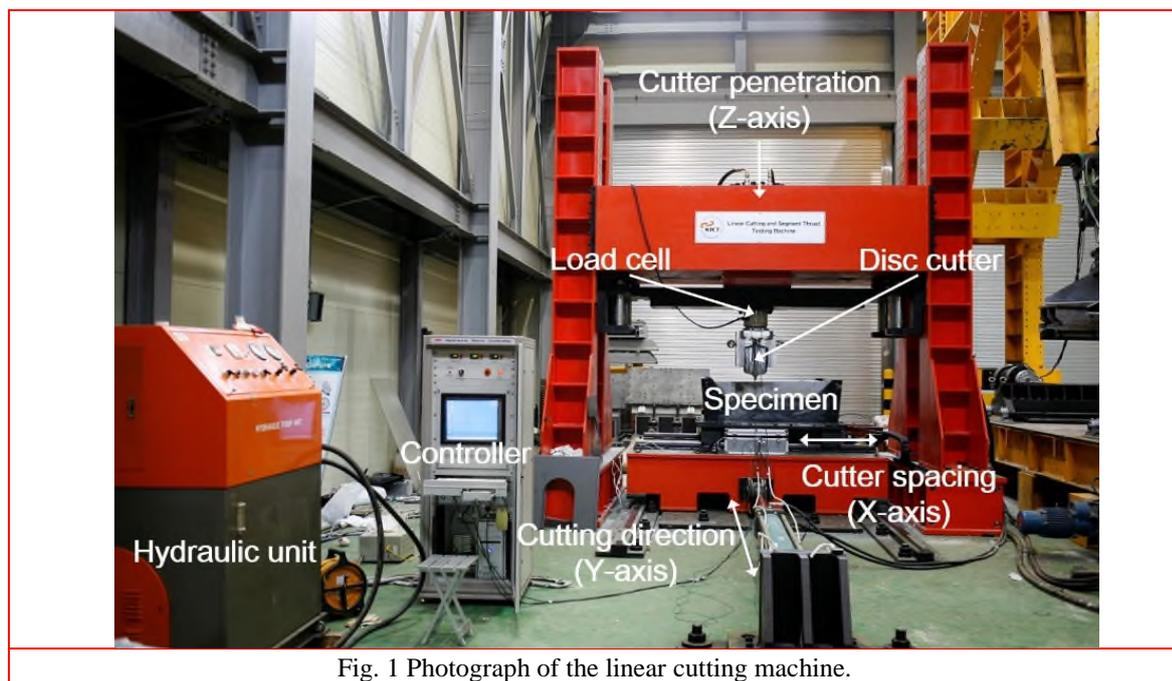
Fig. 1 Photograph of the linear cutting machine.
