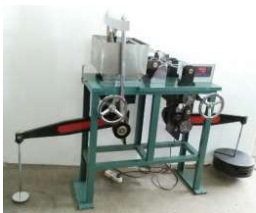
Fig. 1 Photo of the testing apparatus and sketch of the shear box
