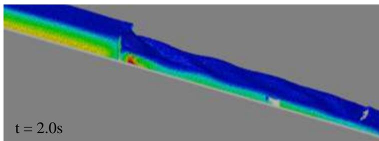
Fig. 7 Time sequence of bridge wash-out simulation by the stabilized ISPH method for initial water height 250mm
