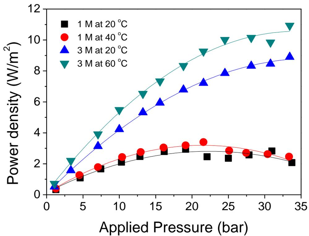
**Figure 7.** Power density as a function of the applied hydraulic pressure for various concentrations of CaCl<sub>2</sub> and temperatures.
