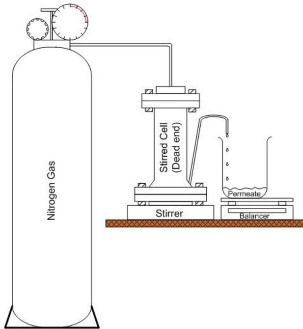
Fig. 2 Experimental set-up of dead-end membrane filtration.
