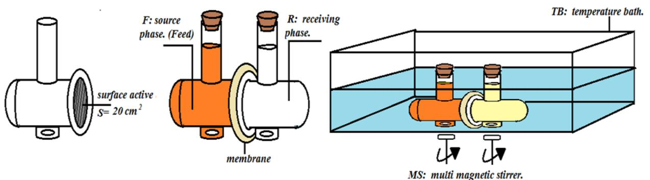
**Figure1: Schema of transport cell.**
