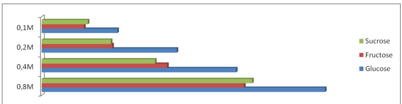
**Figure 3: Evolution of initial flux J0 with the initial substrate concentration relating to facilitated transport of Glucose, Fructose, and sucrose.**
