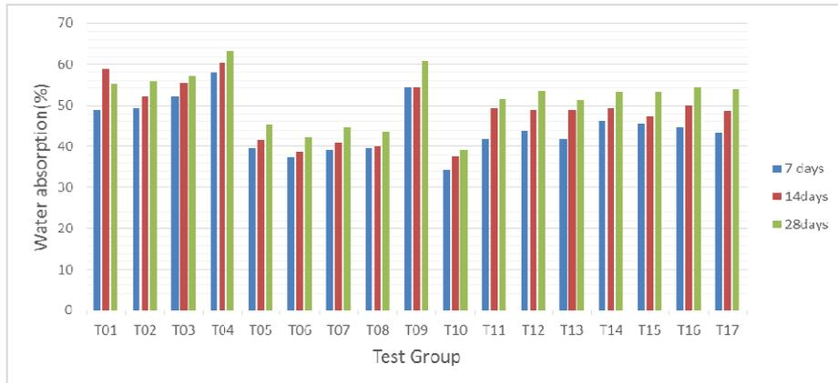
Figure 7 experimental results of water absorption at 7, 14, 28-day for CMFM
