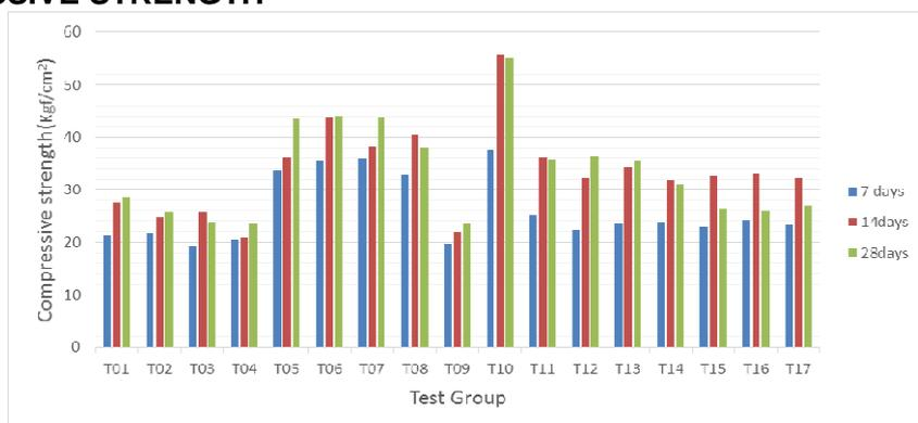
Figure 8 experimental results of compressive strength at 7, 14, 28-day for CMFM
