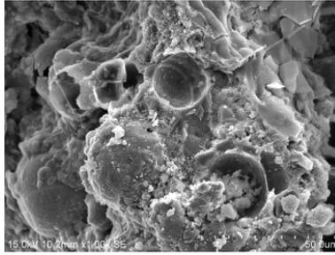
Figure 4 SEM view for cement and inorganic microspheres (1000 times)
