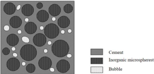
Figure 2 Composition Mechanism of CMFM
