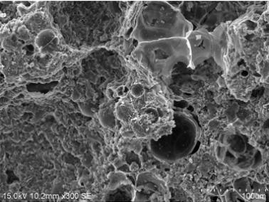
Figure 3 SEM view for cement and inorganic microspheres (300 times)
