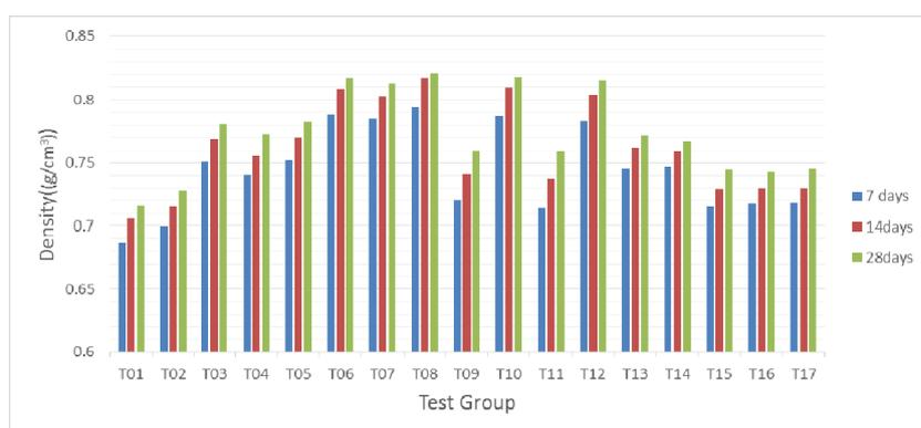
Figure 5 experimental results of density at 7, 14, 28-day for CMFM
