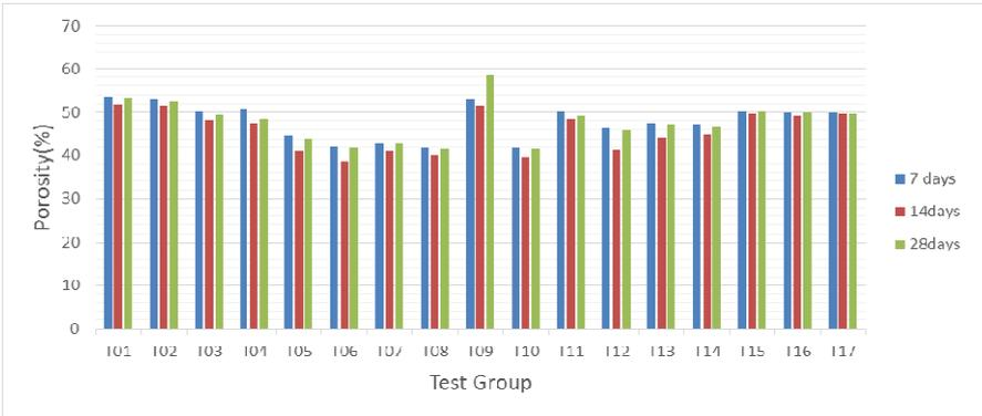
Figure 6 experimental results of porosity at 7, 14, 28-day for CMFM
