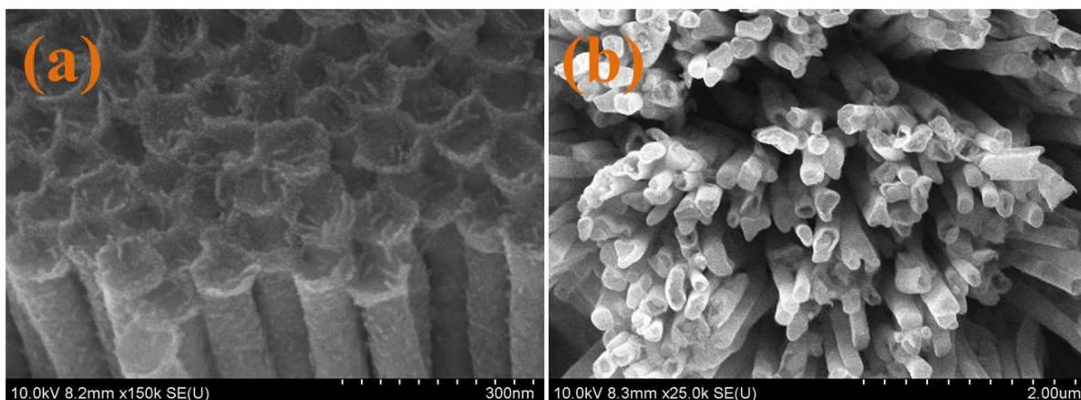
**Figure 2:** (a, b) SEM micrographs of Ni-CoO core-shell nanowires.
