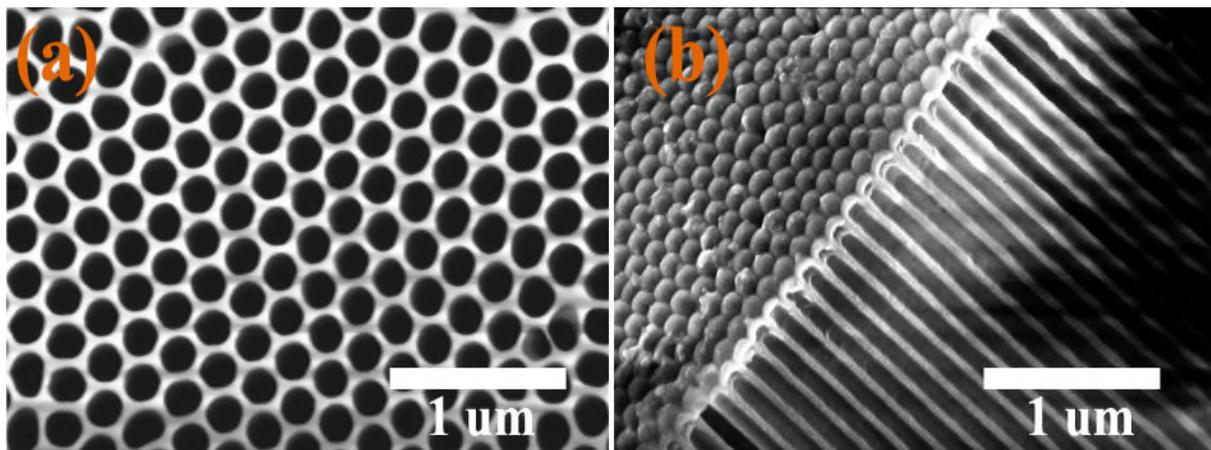
**Figure 1:** (a) Top view of AAO template (b) Cross-sectional view of AAO template taken from SEM.
