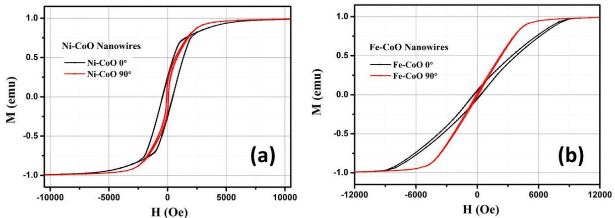
**Figure 3:** Hysteresis loops for (a) Ni-CoO core-shell nanowires (b) Fe-CoO core-shell nanowires, measured with the applied field parallel and perpendicular to the template surface.
