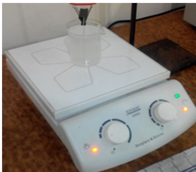
Fig.1 Experimental set up for the deposition of ZnO nanorods
