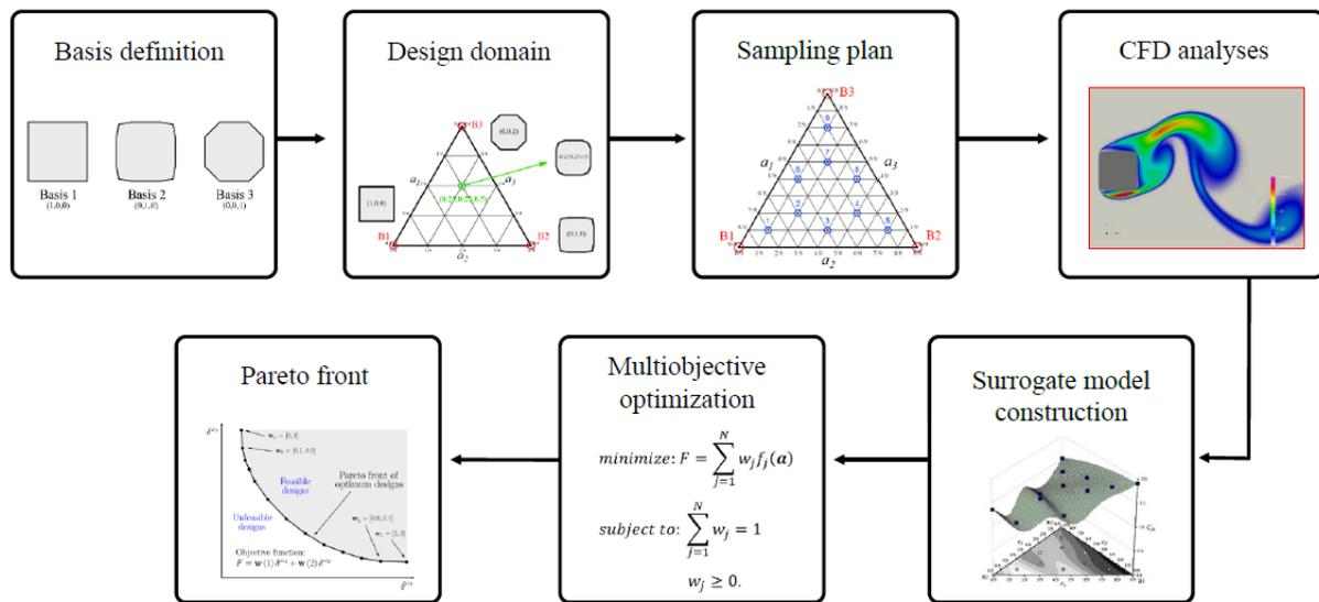
Fig. 1 Multiobjective shape optimization flow chart.
