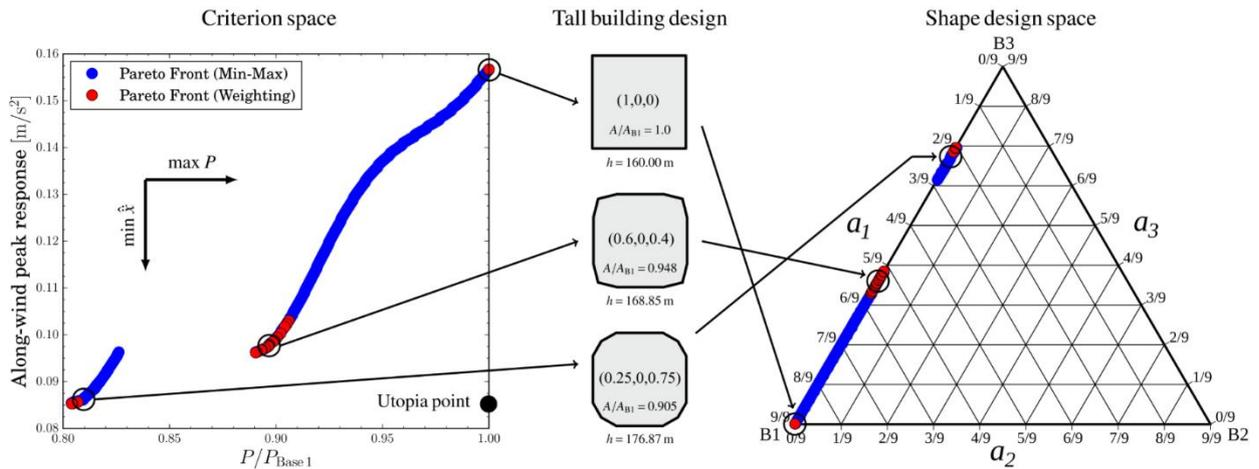
Fig. 3 Pareto optimal set in criterion and design spaces.
