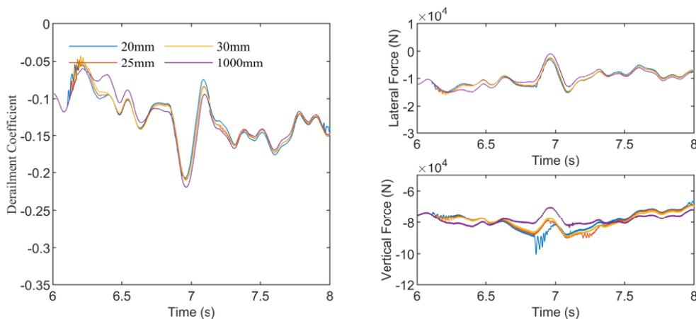
Fig. 4 The wheel response when PGA is 0.3g
