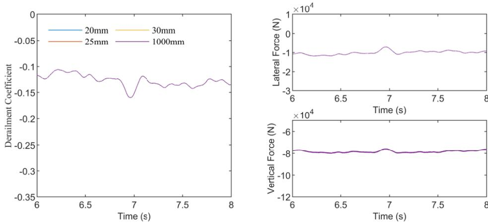
Fig. 3 The wheel response when PGA is 0.1g
