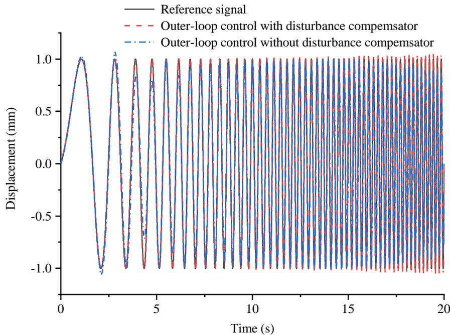
**Fig. 6** Tracking displacements of shaking table for 0.1-5Hz chirp signal
