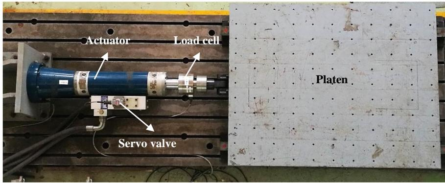
**Fig. 2** The hydraulic shaking table at Central South University
