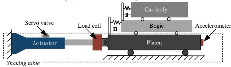
Fig. 5 Uniaxial shaking table fixed with vehicle model
