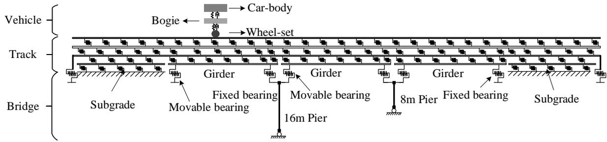
Fig. 4 Model of bridge and train
