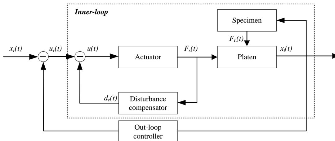
Fig. 1 Framework of disturbance rejection control
