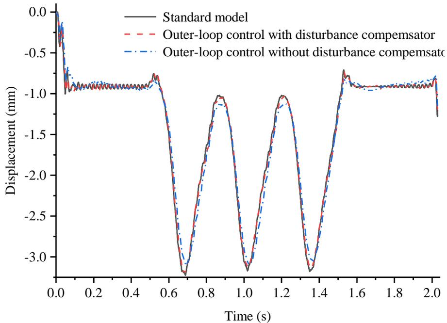
Fig. 7 Response displacement of wheel-set in RTHS
