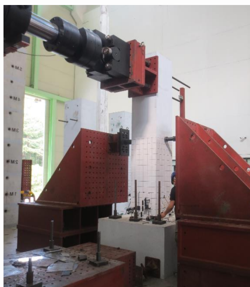
Fig. 2 Setup for lateral loading test
