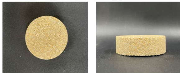
Specimen size Height: 20 mm Diameter: 63 mm
