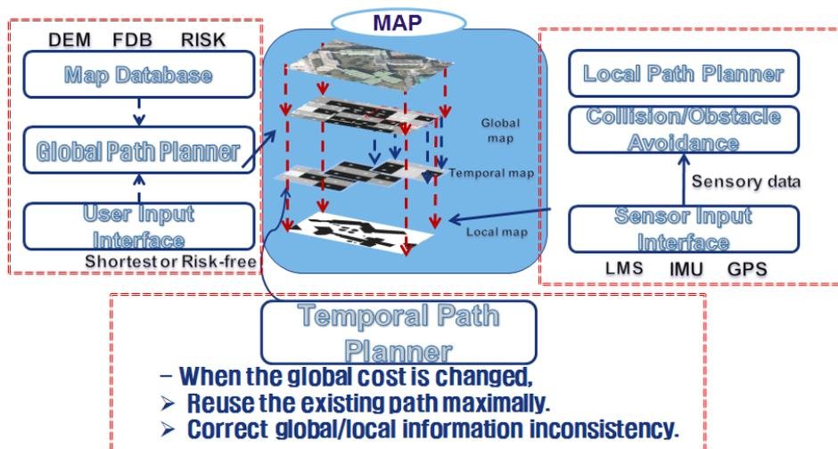
Fig. 4 Integrated path planner for outdoor environment
