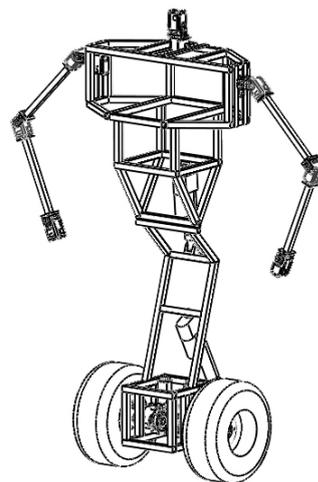
Fig. 3b TeleBot lightweight metal frame angled to maintain TeleBot shape
