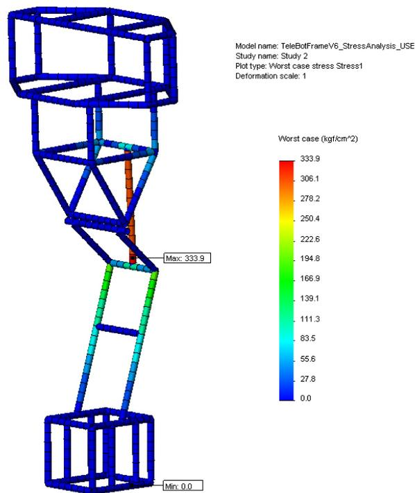
Fig. 6 Weight on upper TeleBot frame – stress analysis of worst case scenario
