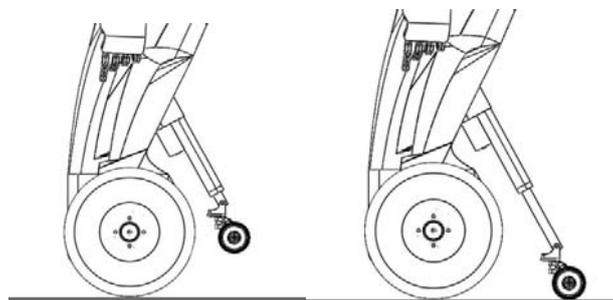
Fig. 4a Retracted linear actuator while TeleBot is in motion on flat ground
