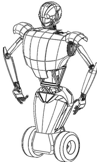
Fig. 3a Modified physical TeleBot exterior with frame for the real world
