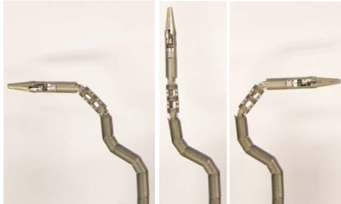
Fig. 4 Bending of the the wrist joint: (a) 90^\circ , (b) 0^\circ , and (c) -90^\circ
