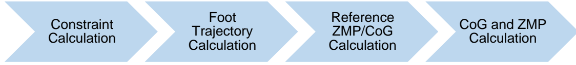
Fig. 5 Real-time trajectory generation system 2
