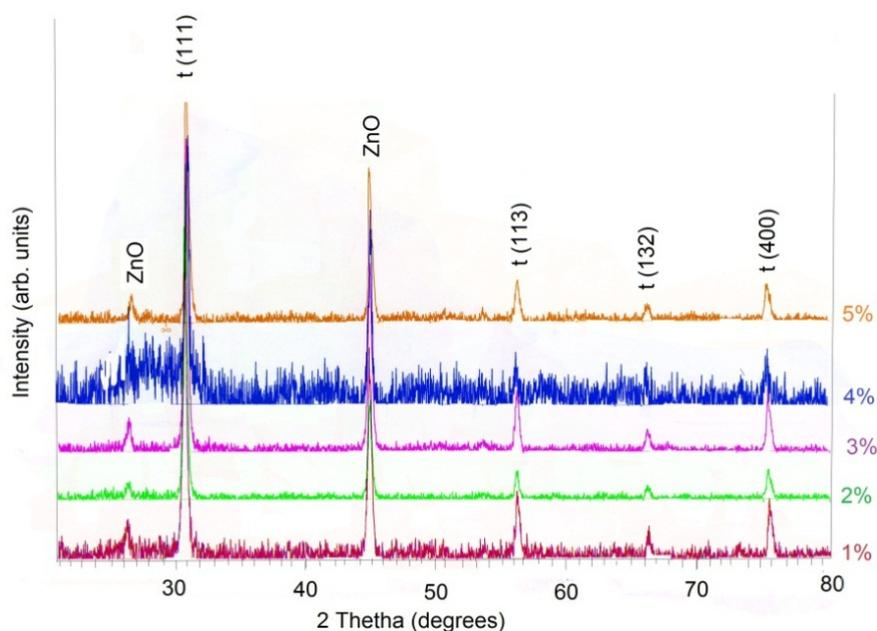
Fig. 3 XRD patterns of  $ZrO_2$ -ZnO nanoparticles in basic medium (pH = 9)
