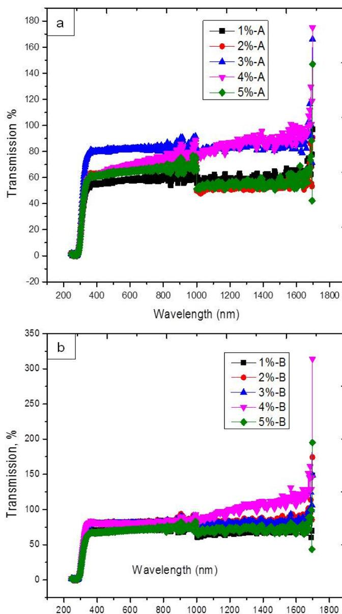
Fig. 5 Transmission plots of ZnO doped zirconia at different concentrations: (a) Acidic (pH = 2) and (b) Basic (pH = 9)
