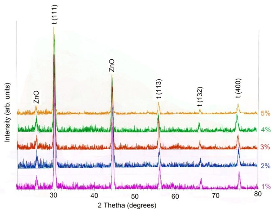
Fig. 2 XRD patterns of  $ZrO_2$ -ZnO nanoparticles in acidic medium (pH = 2)
