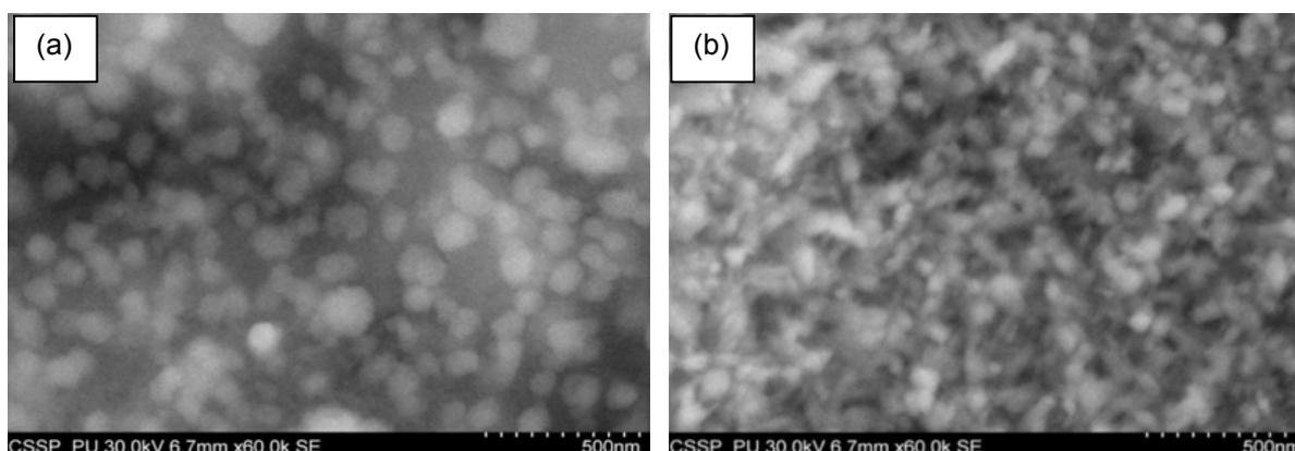
Fig. 4 SEM images of (a) undoped and (b) ZnO doped  $ZrO_2$  nanoparticles
