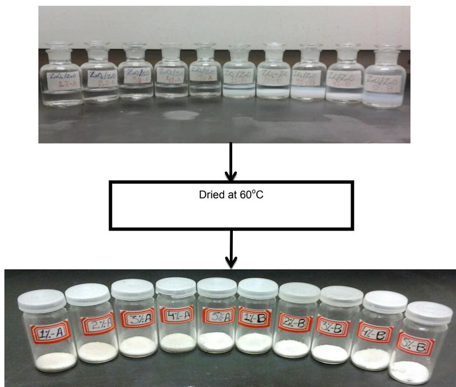
Fig: 1. As-synthesized undoped and ZnO doped  $\text{ZrO}_2$  NPs
