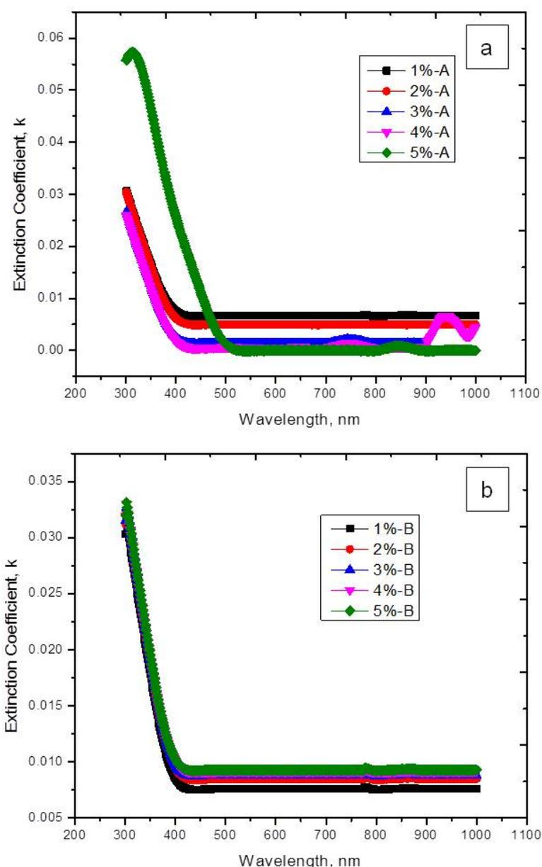
Fig. 8 Extinction coefficient of basic (pH = 9) ZnO-Zirconia as a function of wavelength
