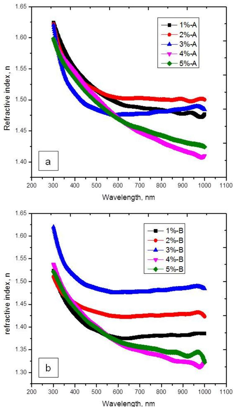
Fig. 7 Refractive index (a) acidic (pH = 2) and (b) basic medium (pH = 9) as a function of wavelength
