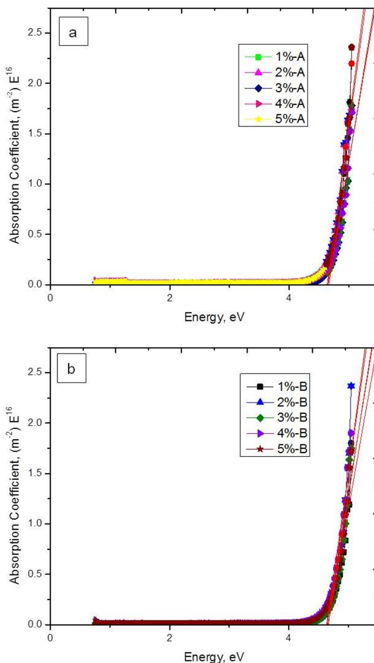
Fig. 6 Band gap of ZnO doped zirconia in (a) acidic (pH = 2); and (b) basic medium (pH = 9)
