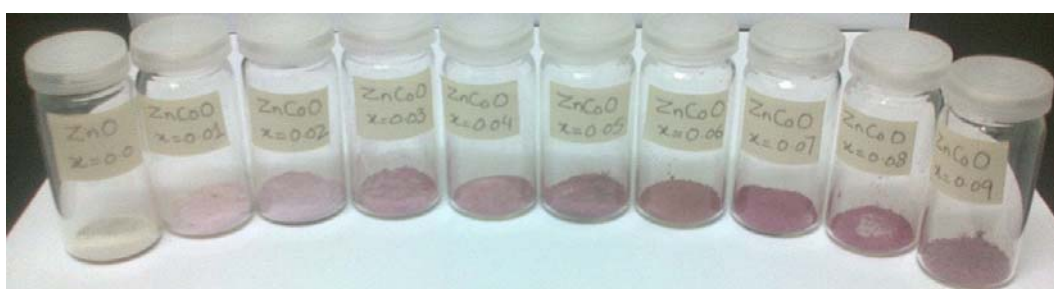
Fig. 2 Co doped ZnO nanopowder with variation from x = 0.00 to x = 0.09
