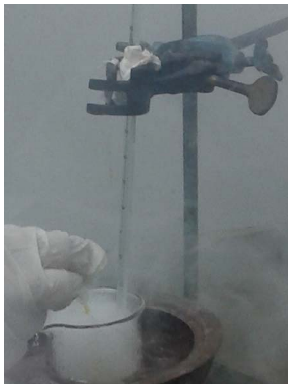
Fig. 1 Experimental setup for TiO 2 nanoparticles showing exothermic reaction during synthesis
