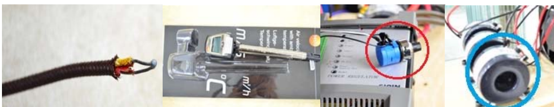
Fig. 3 Thermal couple, wind gauge, variable resistor and current transformer
