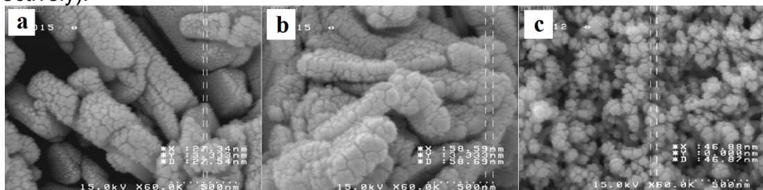
Fig. 3. FESEM photograph of compound 1 nanoparticles prepared by (a) ultrasonic generator 138 W in concentration of initial reagents [Pb^{2+}] = [L^-] = [I^-] = 0.1 M, (b) ultrasonic generator 138 W in concentration of initial reagents [Pb^{2+}] = [L^-] = [I^-] = 0.05 M and (c) ultrasonic generator 305 W in concentration of initial reagents [Pb^{2+}] = [L^-] = [I^-] = 0.01 .
