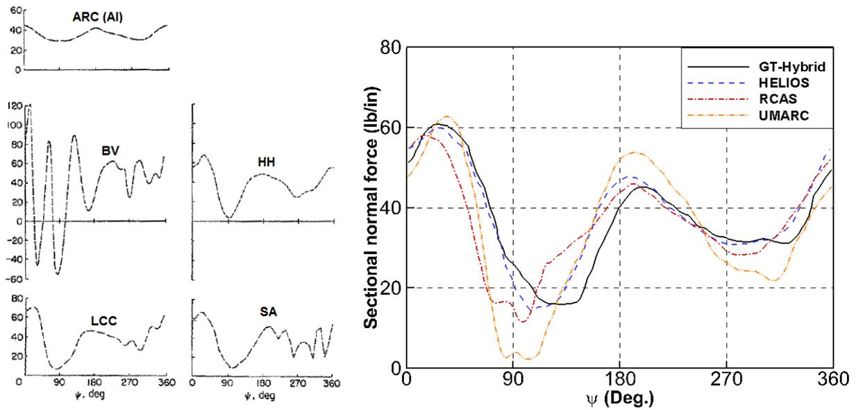
Fig. 6 Comparison of lift and normal force airloads (lb/in.) vs azimuth;  $r=0.8R$
