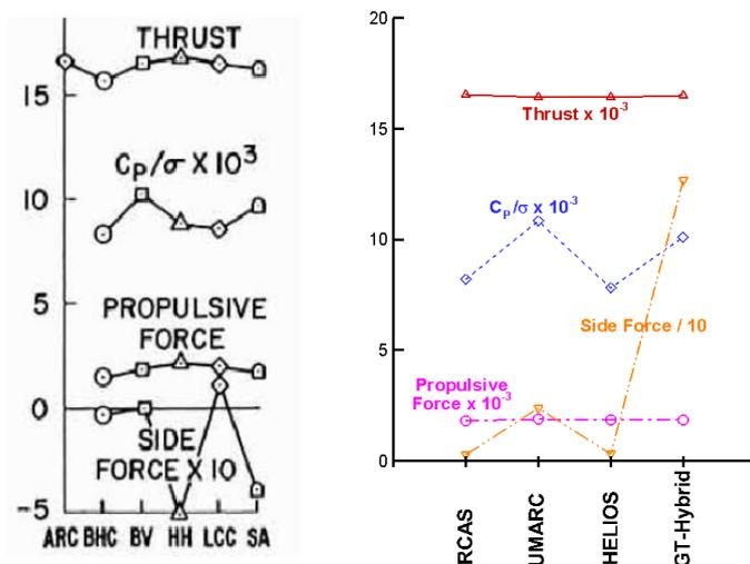
Fig. 5 Comparison of trim rotor forces and power results (Left : 1974, Right : Present)
