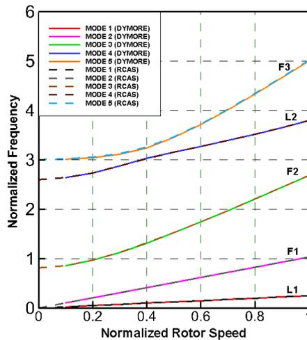
Fig. 4 Comparison of rotating blade natural frequencies (per rev) vs rotor speed
