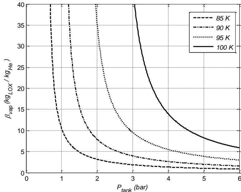
Fig. 6 Variation of evaporation intensity of liquid oxygen into helium bubbles ( $\beta_{vap}$ ) according to the temperature of liquid oxygen and the tank pressure
