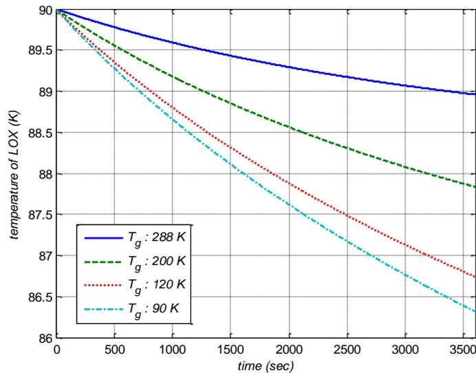
Fig. 5 The temperature variation of liquid oxygen as the Injected helium temperature (at  $\dot{m}_i^{ex} = 0$ ,  $P_t = 2\text{bar}$ ,  $\dot{m}_g = 0.02\text{kg/sec}$ )
