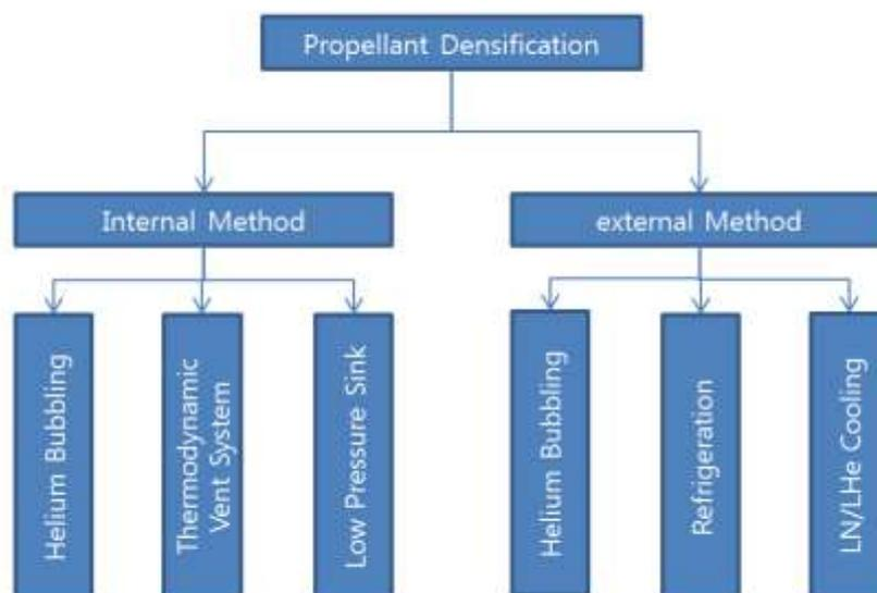
Fig. 1 Propellant densification methods
