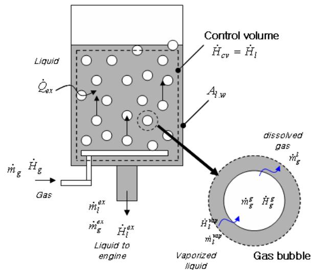
Fig. 2 The schematic of helium injection
