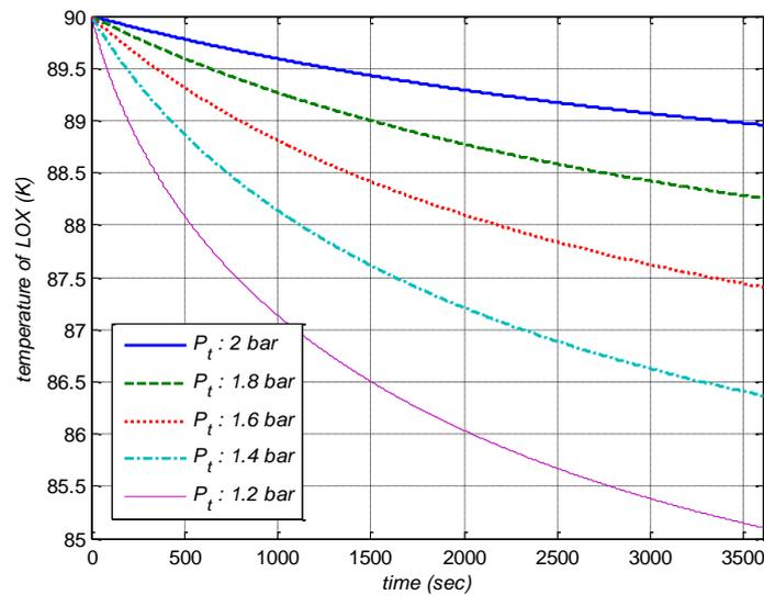
Fig. 4 The temperature variation of liquid oxygen as the pressure of the tank (at  $\dot{m}_i^{ex} = 0$ ,  $T_g = 288K$ ,  $\dot{m}_g = 0.02kg/sec$ )
