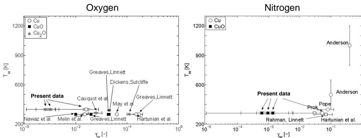
Fig. 1 Variation of surface catalytic efficiency with wall temperature (after Cheung et al. (2015)).
