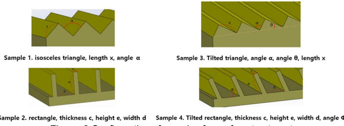
Figure. 2 Configuration of samples for surface treatment
