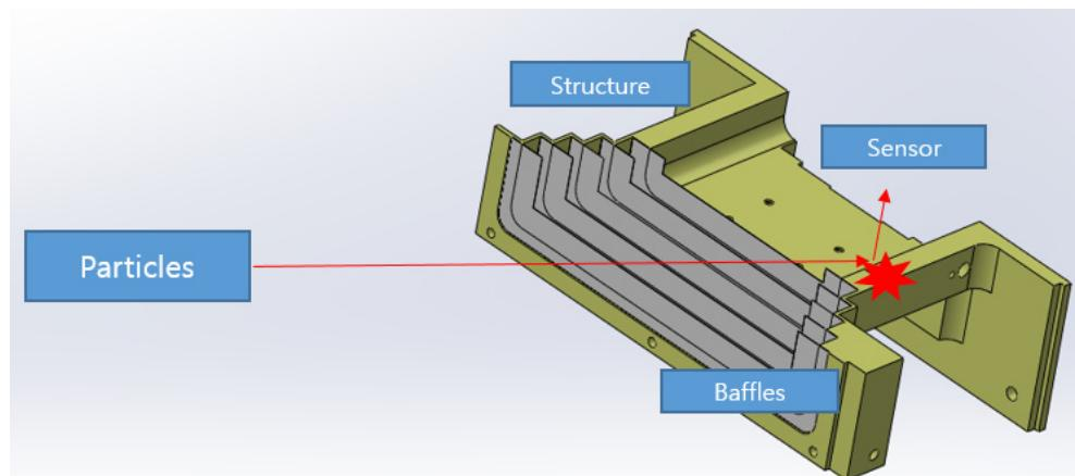
Figure. 1 Configuration of telescope structure and reflected particle incidence
