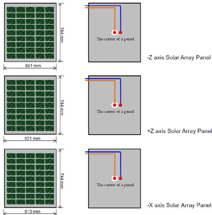
Fig. 1 NEXTSat-1 solar array panels: front side (left) and rear side (right)
