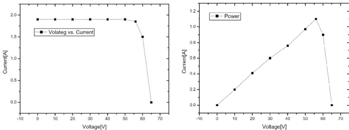
Fig. 2 NEXTSat-1 solar array performance: voltage vs. current (left) and power (right)
