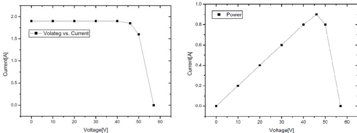
Fig. 3 NEXTSat-1 solar array performance: voltage vs. current (left) and power (right)
