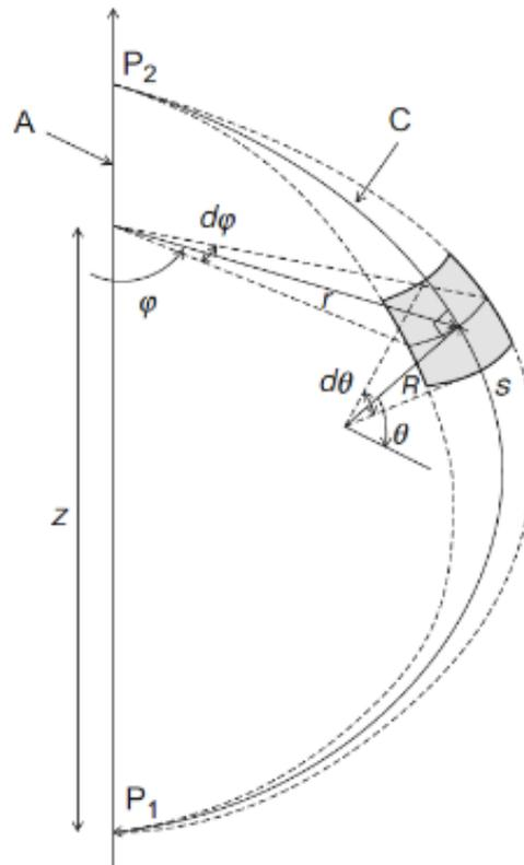
Fig. 1 Surface elements on balloon shape formed by rotating curve C around axis A (Yajima 2004)
