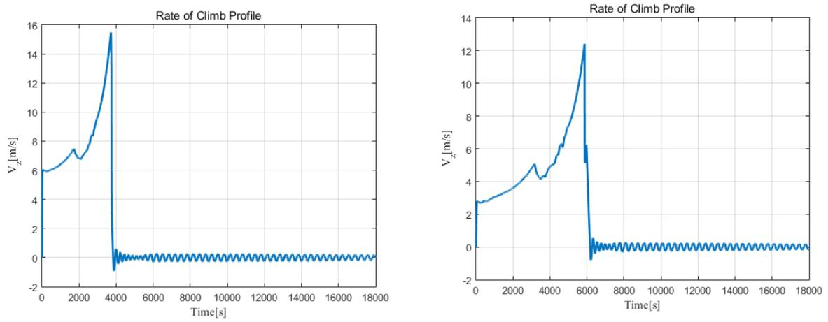
Fig. 9 Rate of climb profile for base and optimized design
