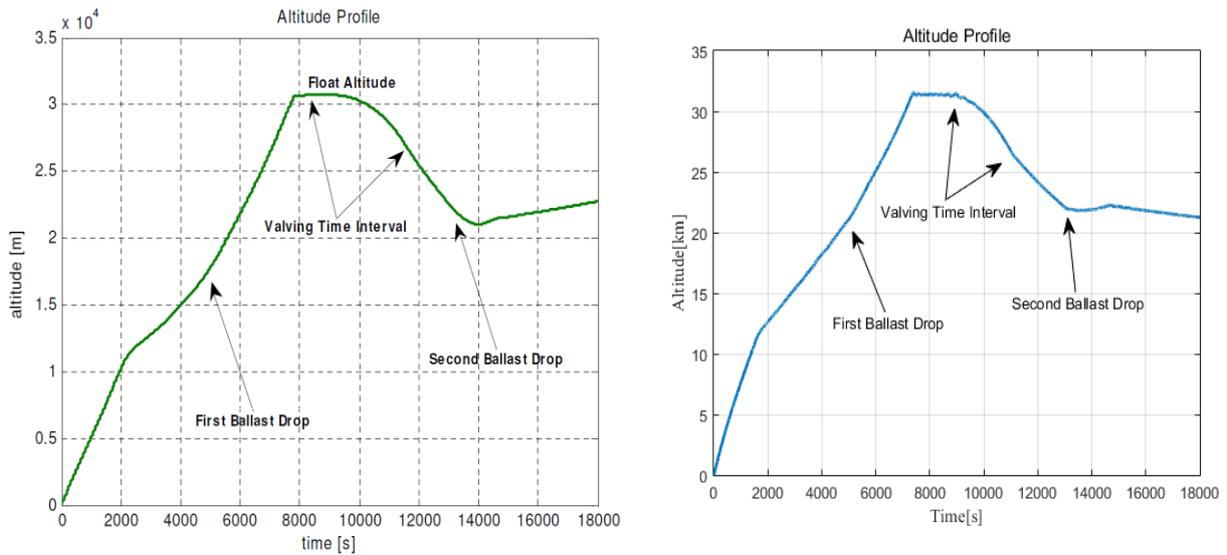
Fig. 3 Altitude vs time data of ACRHAB (left) and our code (right)
