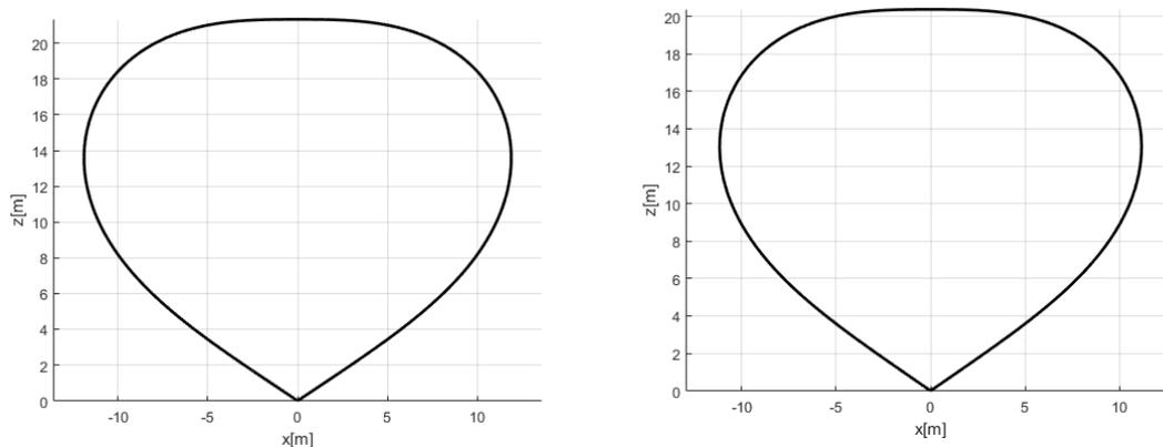
Fig. 7 Natural balloon shape when fully inflated for base and optimized design
