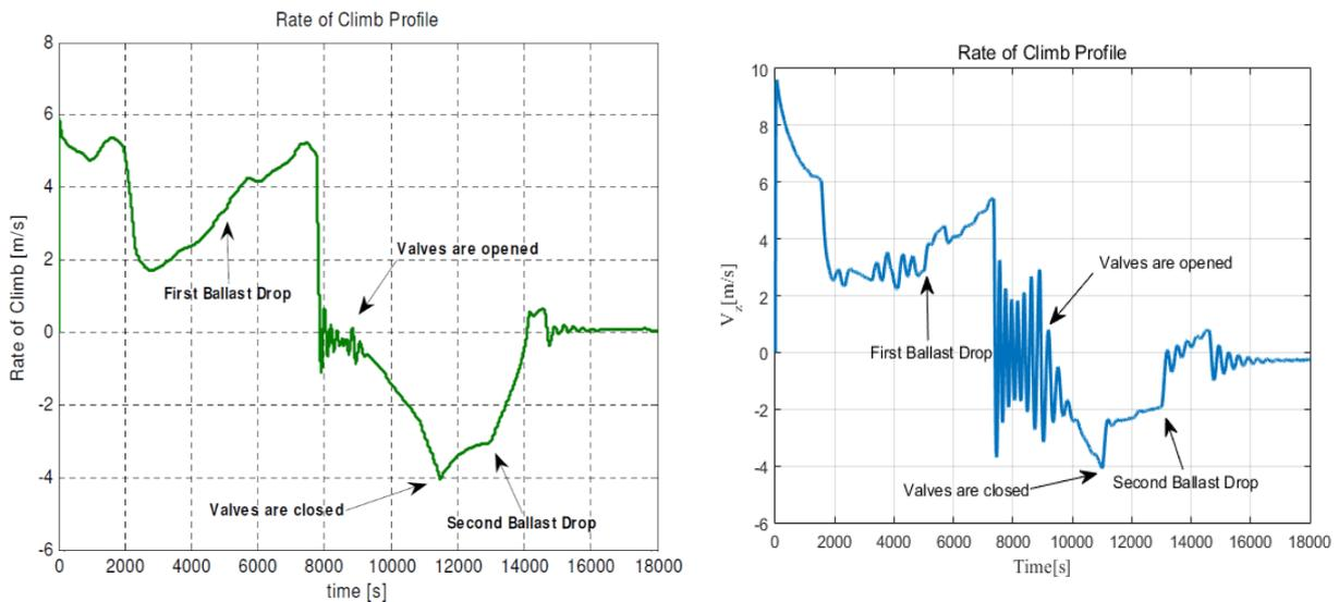
Fig. 4 Ascent rate vs time data of ACHAB (left) and our code (right)
