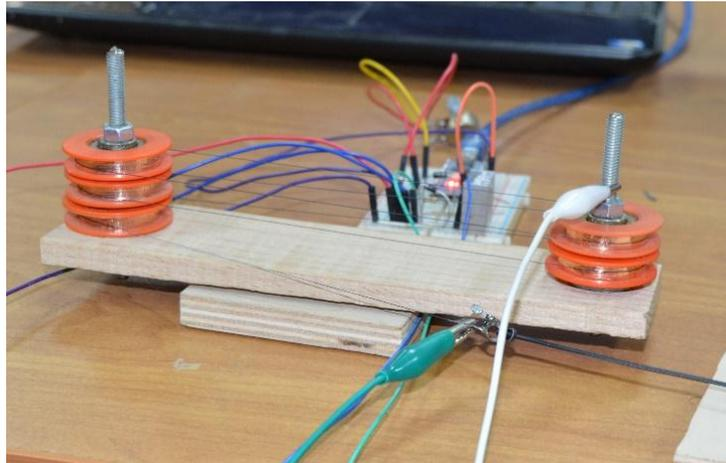
Fig. 17 Final form of the SMA actuator.
